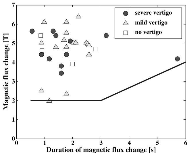
**Fig. 1.** The vertigo threshold in terms of magnetic flux density change,  $\Delta B$ , plotted as a function of duration of a head shake or nod inside a 7 T MR scanner (Glover et al. 2007). The two line segments show the basic restriction for magnetic flux change during any 3 s period during the movement (see Recommendations).
