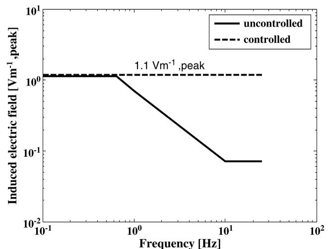
**Fig. 2.** Basic restrictions for the induced electric field for uncontrolled and controlled exposure conditions. The basic restrictions for uncontrolled exposures are based on protection against magnetophosphenes and peripheral nerve stimulation. The basic restrictions for controlled exposures are based on protection against peripheral nerve stimulation only. Above 1 Hz, the basic restrictions are equal to the occupational basic restrictions in ICNIRP (2010).
