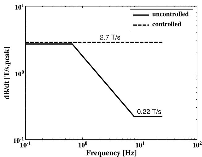
**Fig. 3.** Reference levels for dB/dt for uncontrolled and controlled exposure conditions. Above 1 Hz the reference levels are equal to the occupational reference levels for magnetic flux density (ICNIRP 2010) converted to the peak dB/dt by using (eqn 5).
